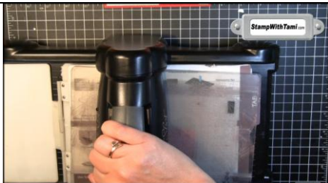
Place on Tab 1 of the multi purpose cutting platform and run through the Big Shot machine
